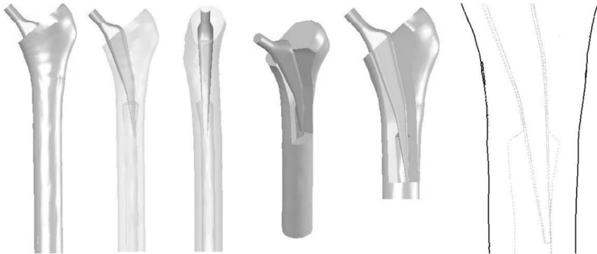
**Figure 6:** Computational geometric model for the implanted femur with the conservative stem.
