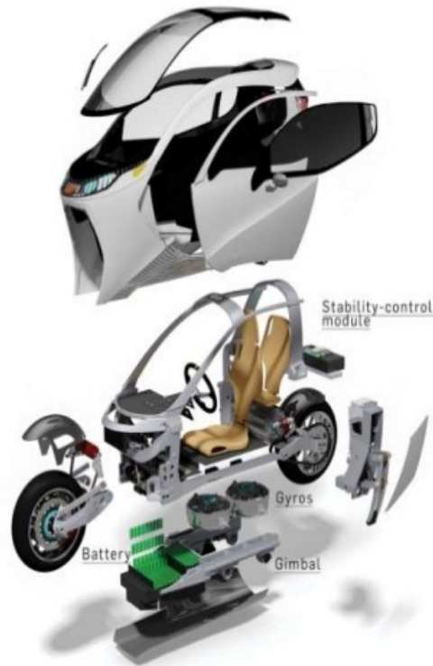
Fig.8: Lit motors concept bike(Exploded Image)
