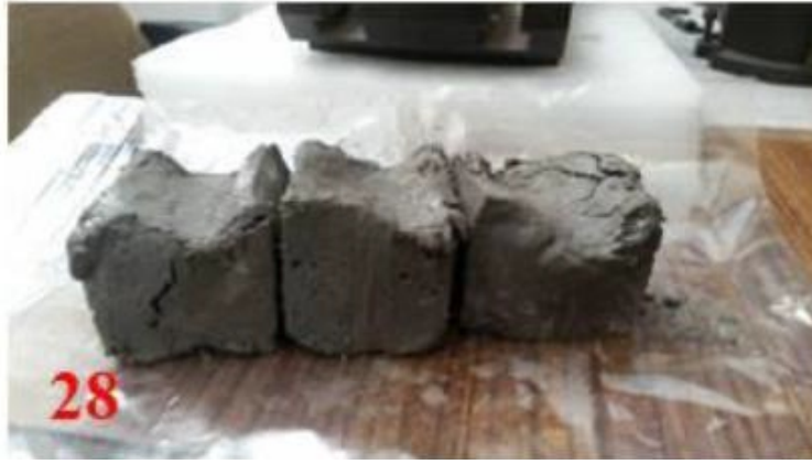
Fig.5. Specimens cured at -20°C that did not harden. From top: 1, 7, and 28 days of curing.
