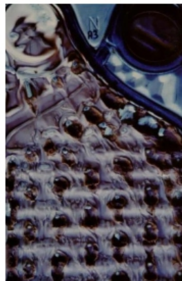
Figure 2 - Reaction Fouling (Protein Deposition) on a Plate and Frame Exchanger Plate
