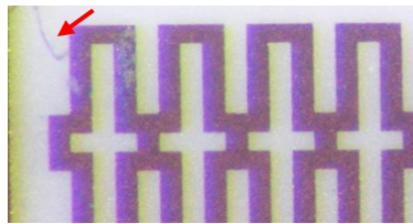
Figure-7: Localized Melting of Resistive Tracks of the Degraded Resistor R4
