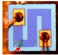
Figure-9: Discontinuity of thin Film track of resistor R6
