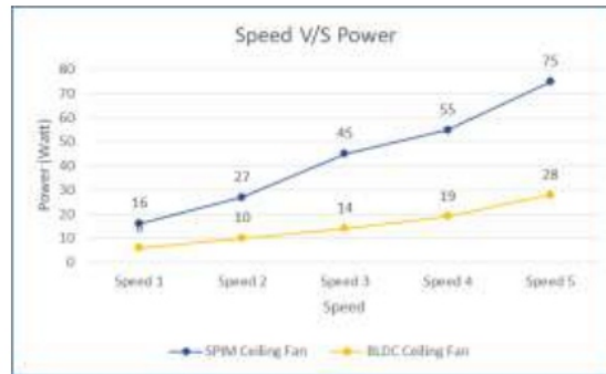
Figure 11. Speed V/S Power consumption by SPIM and BLDC ceiling fan
