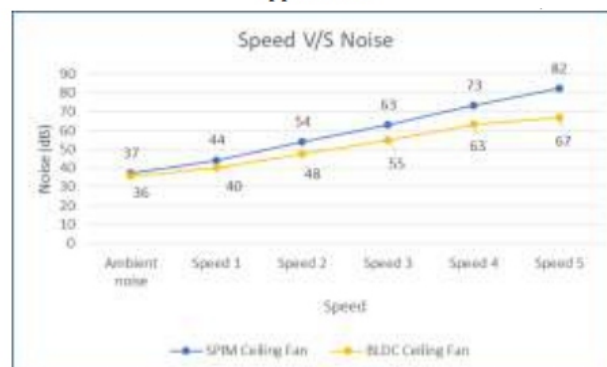
Figure 8. Speed V/S Noise (dB) consumption by SPIM and BLDC ceiling fan.
