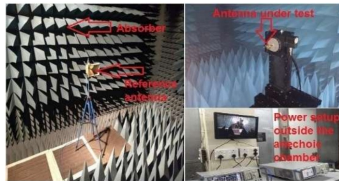
Figure 6: Measurement setup for gain, axial ratio and radiation pattern of the proposed antenna in anechoic chamber
