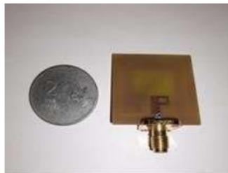
Figure 2(a): Topview of the fabricated antenna
