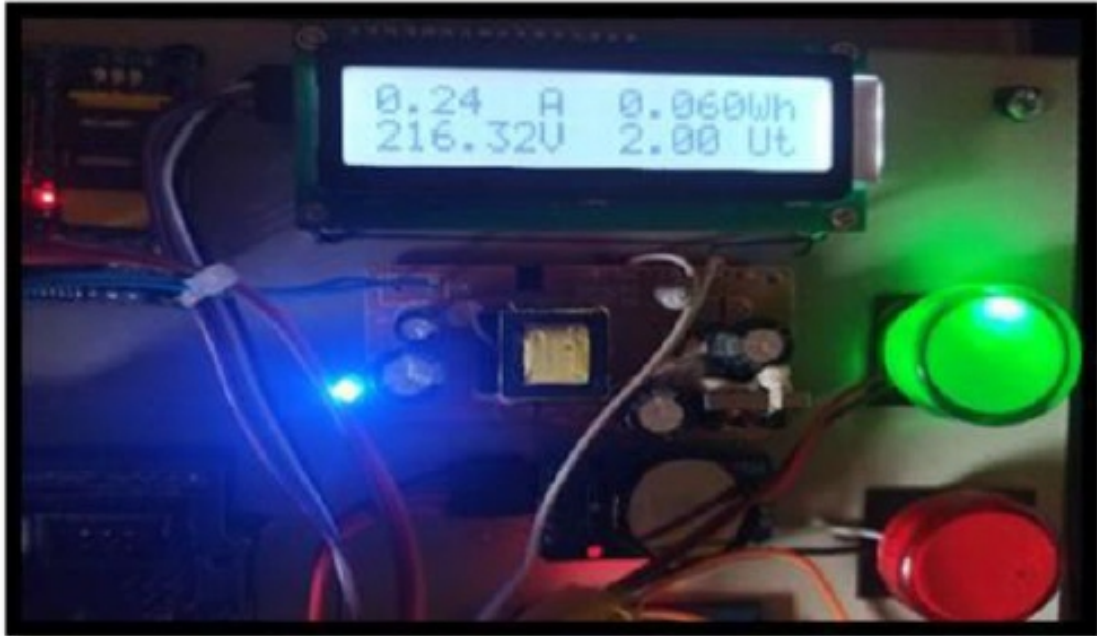
Figure:6(a) The amount of electricity consumption of load displayed on LCD
