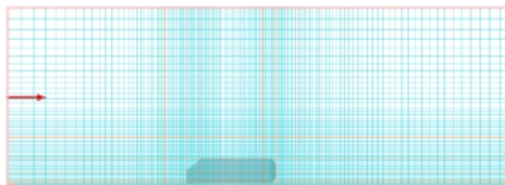
Fig. 5 Optimized grid in the numerical domain ( 162 \times 94 \times 60 )
