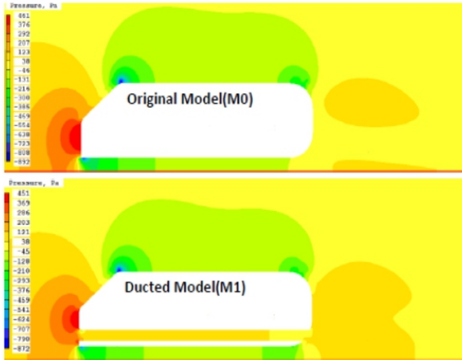
Fig. 6 Pressure distribution on M0 and M1 at 100km/h
