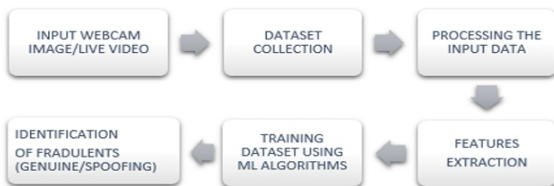
Figure 2. Process Flow Diagram
