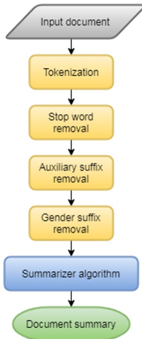
Figure. 1: Block diagram of the extractive text summarization architecture
