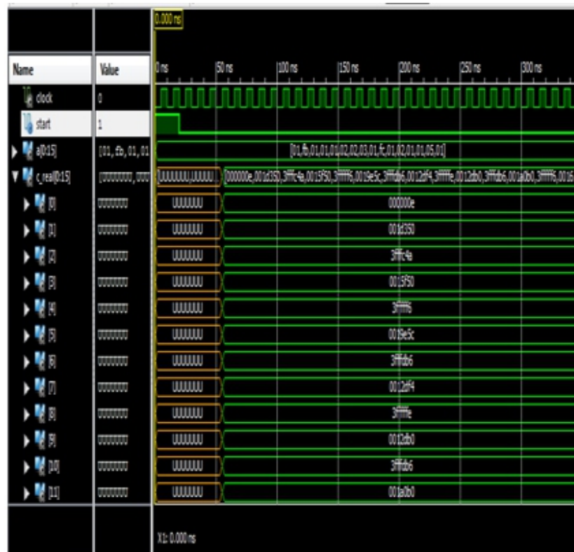
Figure 5: VHDL simulation result for 16 point FFT Algorithm
