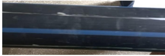
Figure 3. The PE100 polyethylene pipe used for the multiple stress test
