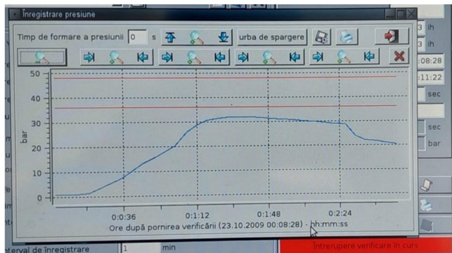
Figure 19. Pressure-time diagram (bar – s) for PE100 polyethylene pipe evaluated under internal pressure test stage
