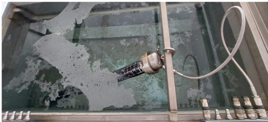
Figure 14. Internal pressure testing of the pipe
