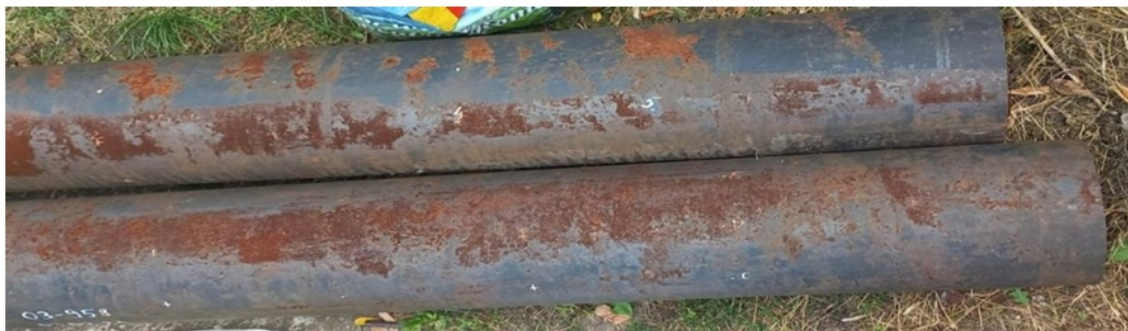
Figure 5. Metal tubes used to simulate the load due to street traffic
