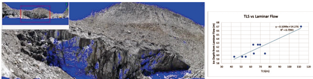
Figure 7 Correlation between TLS ground Measurements and Laminar Flow Model at snout and the Actual Scan of the snout during field visit (15-17 September 2014)
