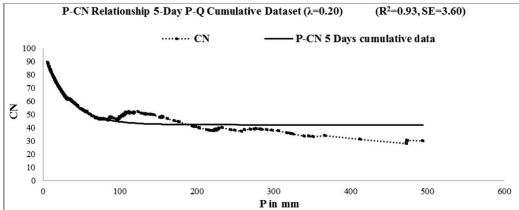
**Figure 3** Comparison of  $P$ - $CN$  relationship, with approximation of asymptotic functions  $CN(P)$  by Equations (7) and (8) for 5 days cumulative  $P$ - $Q$  dataset of Ozat watershed ( $\lambda=0.20$ )
