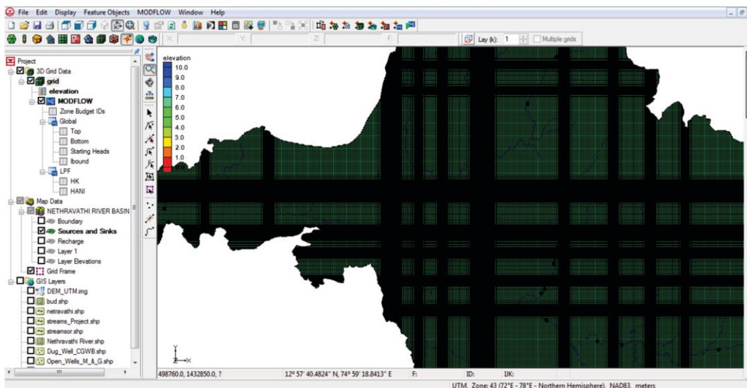
Figure 4 Grid-based MODFLOW numerical model
