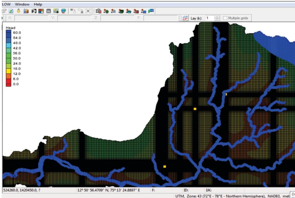
**Figure 6** Groundwater head contours and flow budget of simulated MODFLOW numerical model
