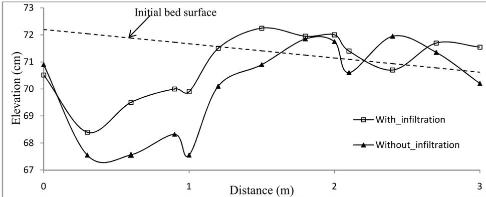
**Figure 6.** Transient bed profiles in the sand bed for 75 minutes.
