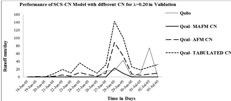
**Figure 4** Performance of SCS-CN Model with Tabulated CN, AFM CN and MAFM CN at daily time scale in validation period (June-July, 2005) for Ozat watershed ( $\lambda=0.20$ )
