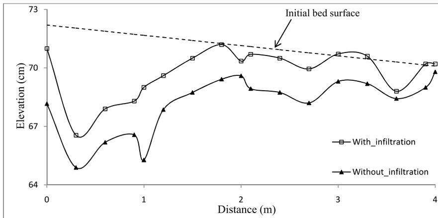
**Figure 7.** Transient bed profiles in the sand bed for 120 minutes.
