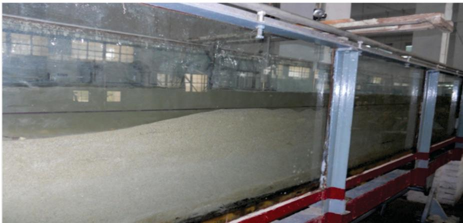
**Figure 4.** A view of degradation channel
