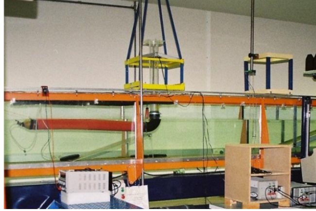
Figure 1: Distensible-tube wave attenuator over a sloping bottom in the wave-flume.
