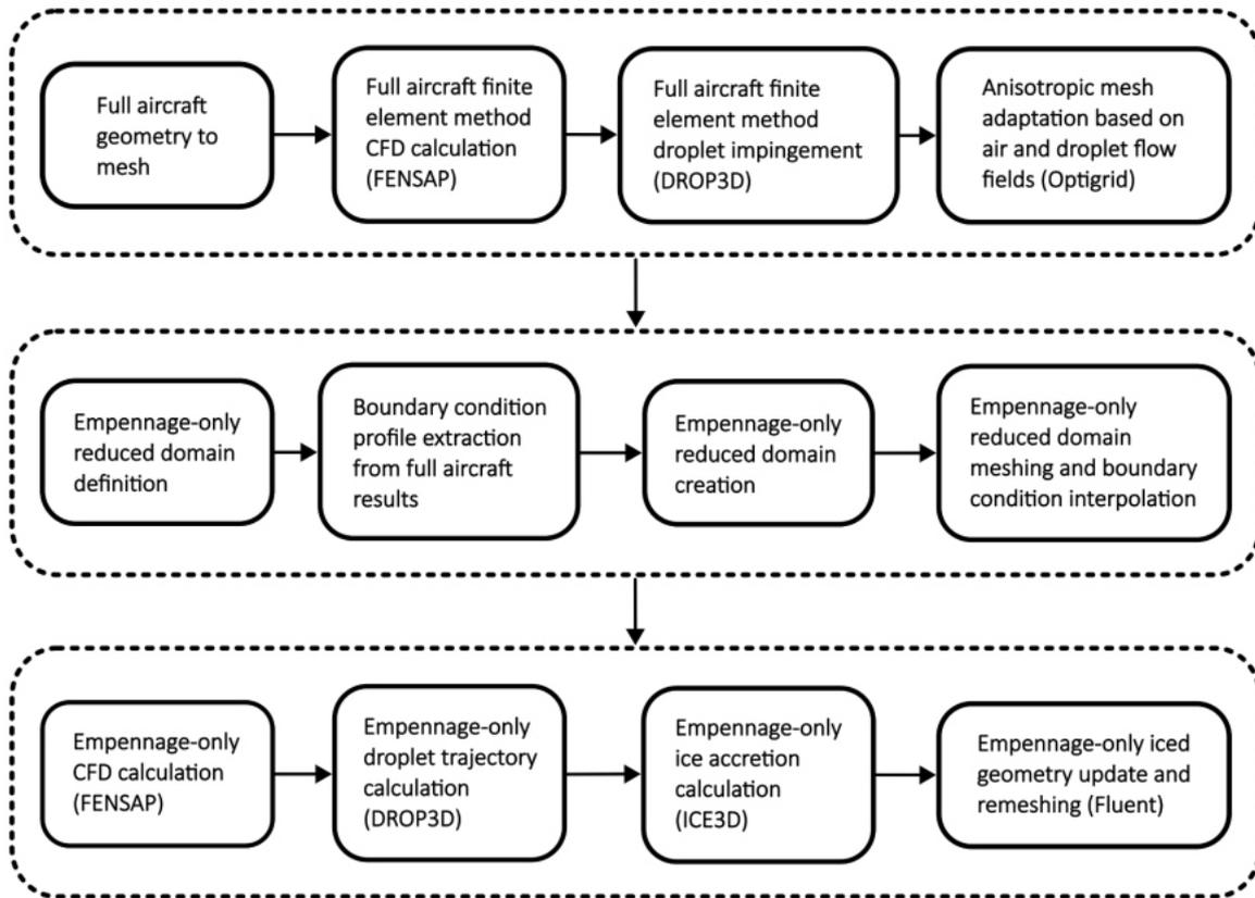
Fig. 9. Flow diagram summarizing the workflow for full aircraft-based empennage inflight icing simulation.
