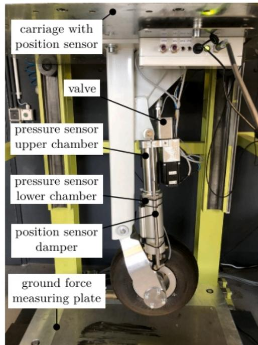
**Fig. 3.** Drop test bench of HEGGEMANN AG with a mechatronic shock absorber integrated into a trailing arm suspension.
