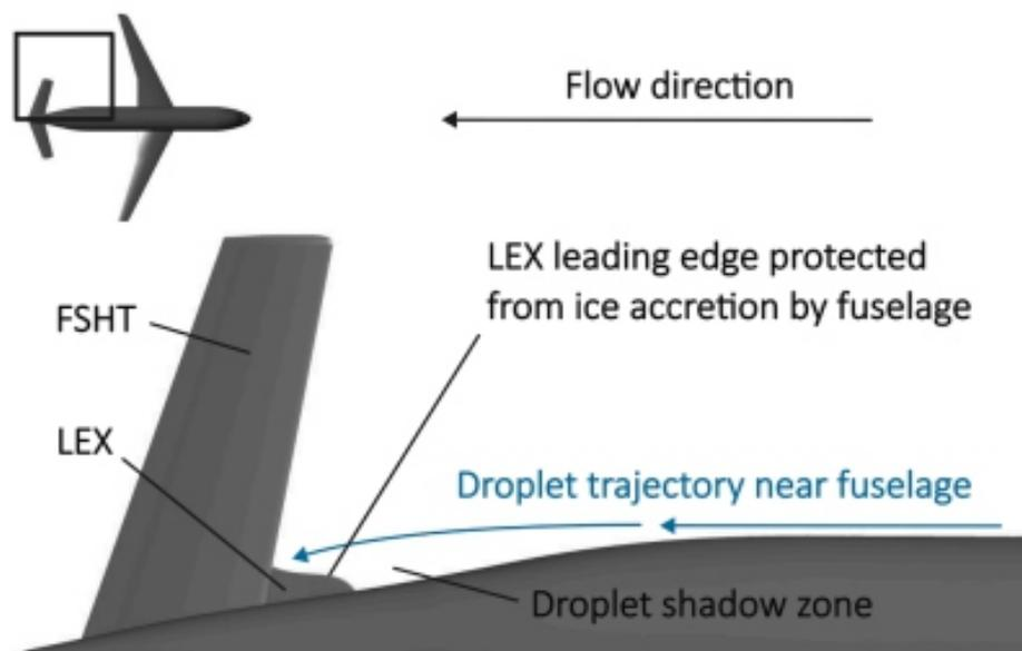
**Fig. 2.** FSHT combined with a LEX located in a droplet shadow zone. This figure has been adapted from [18] with permission, © 2023 SAE International.
