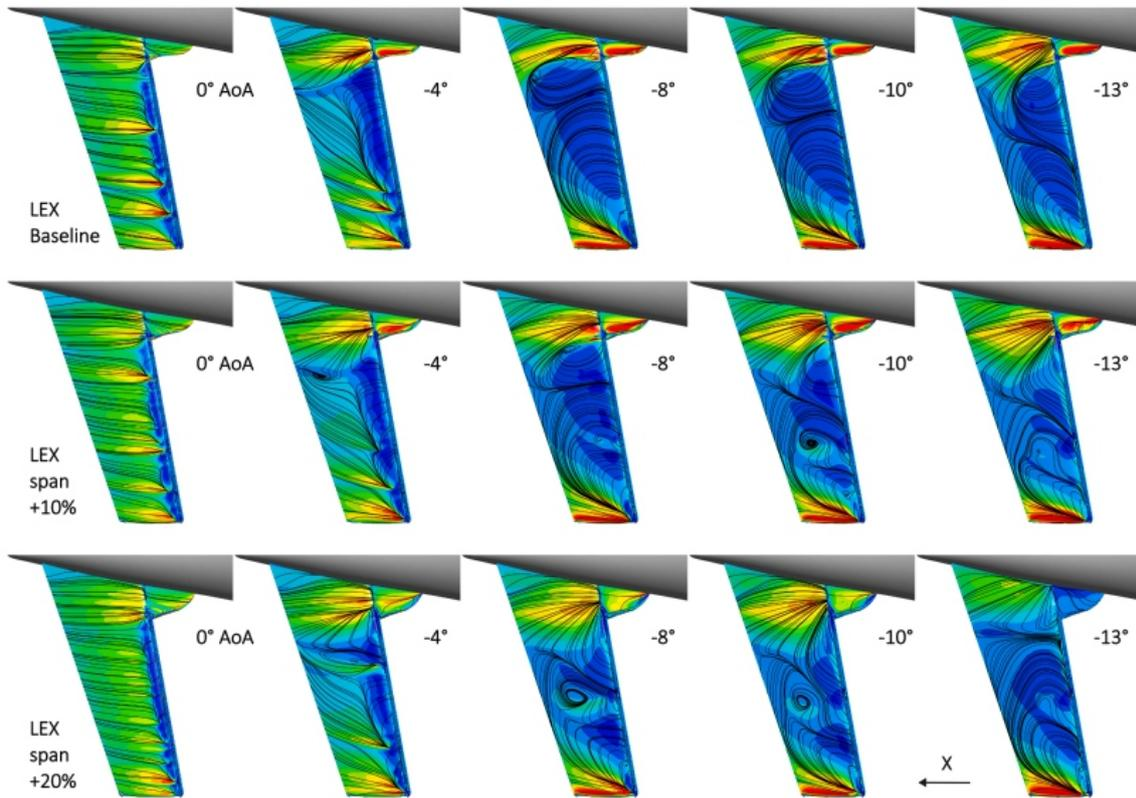
Fig. 38. Suction (lower) surface WSS<sub>x</sub> colour plot, with the same scale as used throughout this paper, with surface WSS vector-based streamlines. The rows are the iced 10° FSHTs with baseline, plus 10 % span, and plus 20 % span LEXs. The columns are 0°, -4°, -8°, -10°, and -13° AoA.
