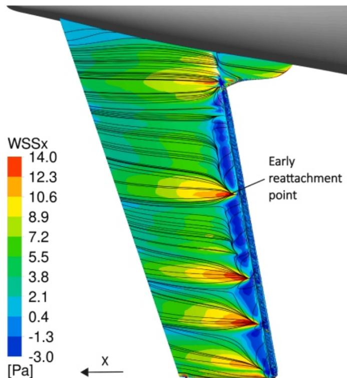
**Fig. 13.** Iced 10° FSHT suction (lower) surface WSS<sub>x</sub> colour plot with surface WSS vector-based streamlines, at 0° AoA. This figure has been adapted with permission from [18], © 2023 SAE International.
