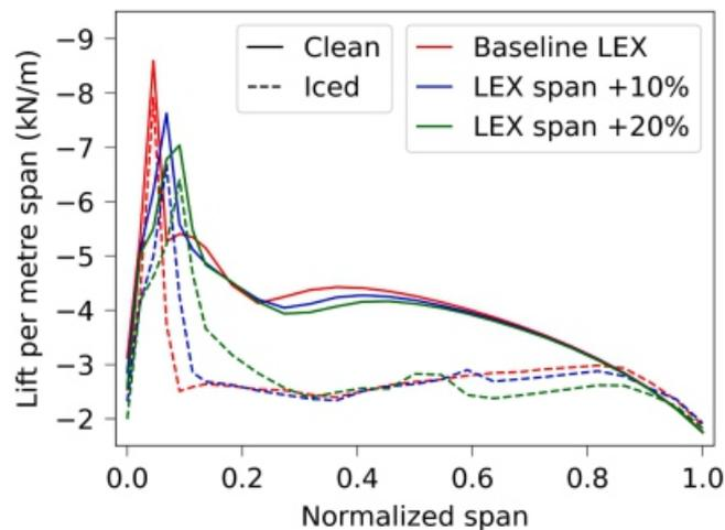
Fig. 39. Spanwise distribution of lift in the form of the integral of streamwise surface static pressure cuts, at -8° AoA.
