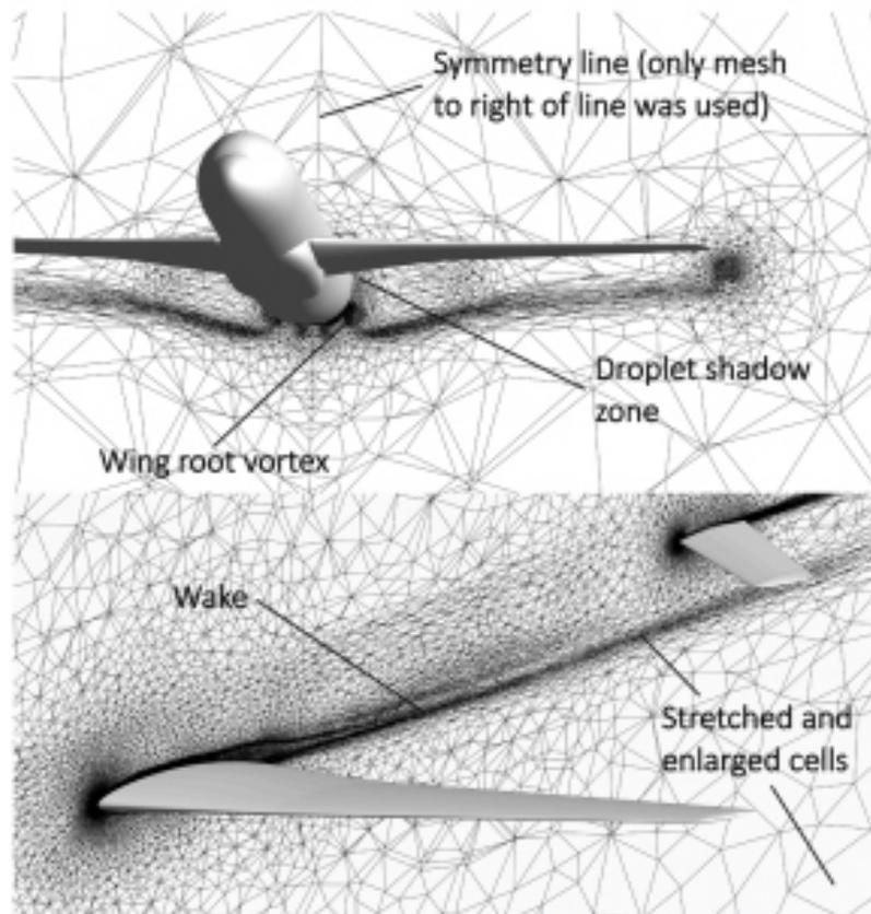
**Fig. 7.** The results of anisotropic adaptation of the volume mesh based on the air and droplet flow solutions. This figure has been adapted with permission from [18], © 2023 SAE International.
