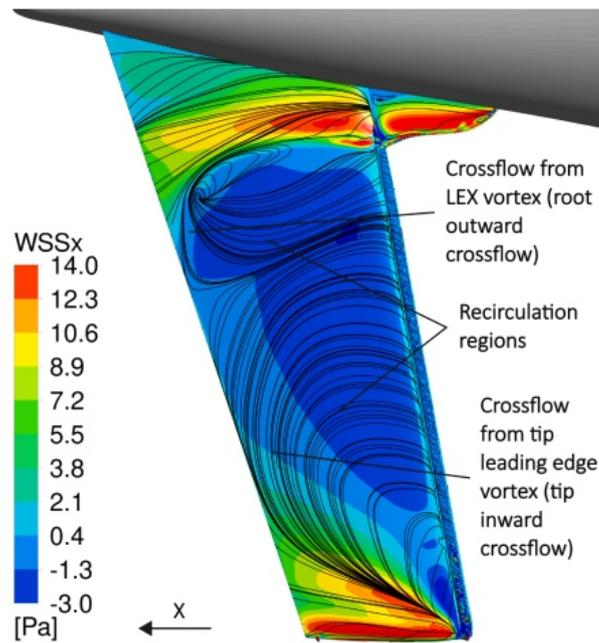
Fig. 18. Iced 10° FSHT suction (lower) surface WSS<sub>x</sub> colour plot with surface WSS vector-based streamlines, at -8° AoA. This figure has been adapted with permission from [18], © 2023 SAE International.
