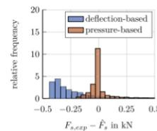
Fig. 8. Stationary load estimation error for the pressure-based and deflection-based approaches for a total of 3,000 different drop tests and a load bin width of 0.05 kN. The brown bars represent the intersection of blue and orange bars.
