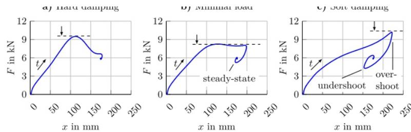
Fig. 1. Force response of the landing gear suspension as a function of the suspension deflection for (a) too hard damping configuration, (b) minimal load damping configuration, and (c) too soft damping configuration for a specific impact scenario.
