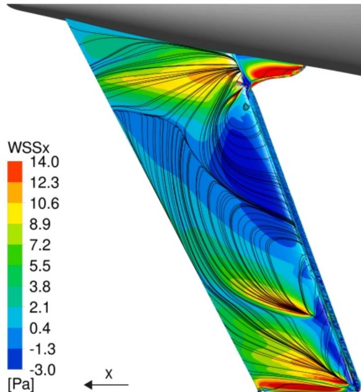
**Fig. 20.** Iced 20° FSHT suction (lower) surface  $WSS_x$  colour plot with surface  $WSS$  vector-based streamlines, at  $-8^\circ$  AoA. This figure has been adapted with permission from [18], © 2023 SAE International.
