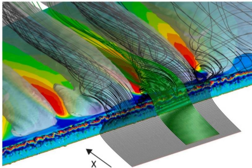
**Fig. 17.** Three dimensional visualization of early reattachment points on the suction surface of the 20° FSHT at -4° AoA. There are WSS<sub>x</sub> surface contours on the same scale as in Fig. 16, a turbulent viscosity isosurface, black streamlines impinging on the leading edge ice, and green streamlines 3 cm below (above in the image).
