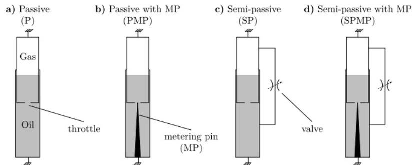
Fig. 2. Investigated passive oleo-pneumatic shock absorber with (a) and without metering pin (b). Investigated semi-passive oleo-pneumatic shock absorber with (c) and without metering pin (d).
