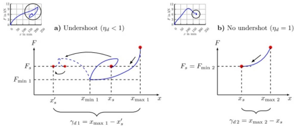
Fig. 5. Comparison of the decompression phases of a soft-damping configuration (a) with that of a hard-damping configuration (b).
