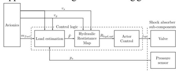
Fig. 6. Semi-passive single action control network of the SP and SPMP variants.
