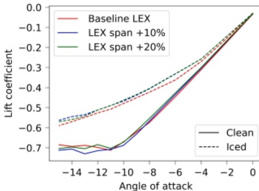
**Fig. 37.**  $C_L$ - $\alpha$  curves for the clean and iced  $10^\circ$  FSHTs baseline, plus 10 % span, and plus 20 % span LEXs.
