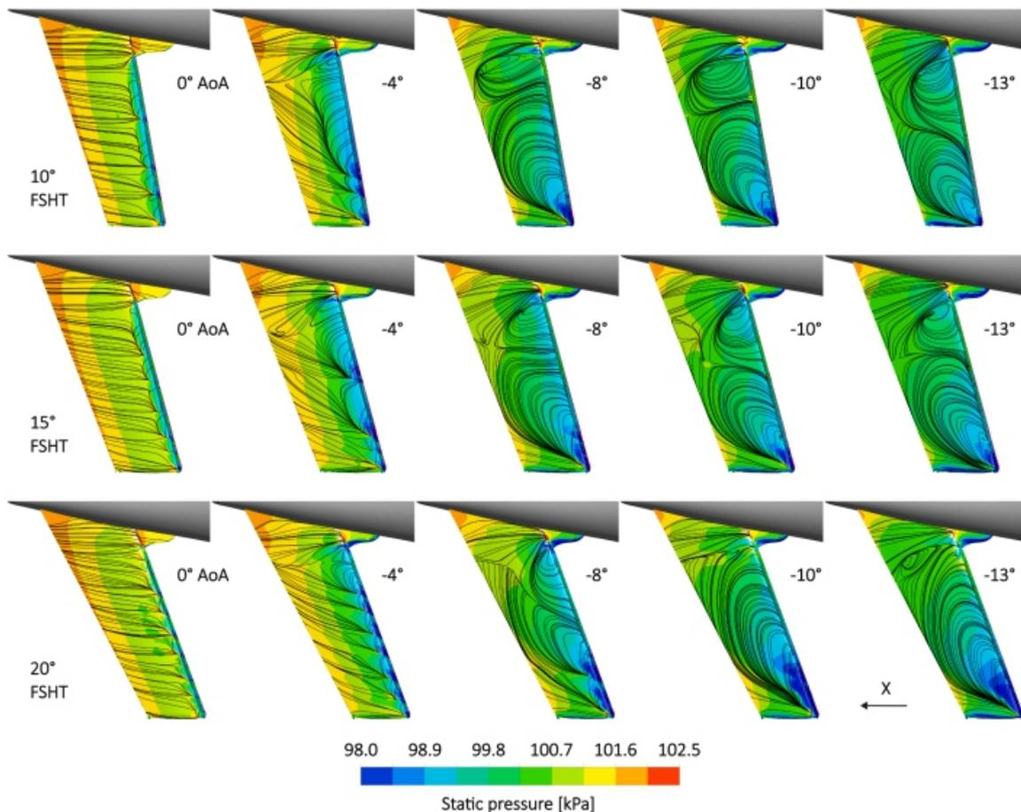
Fig. 24. Suction (lower) surface static pressure colour plots with surface WSS vector-based streamlines. The rows are iced 10°, 15°, and 20° FSHTs. The columns are 0°, -4°, -8°, -10°, and -13° AoA.
