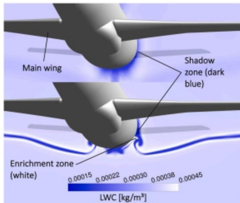
**Fig. 8.** LWC distribution before (top) and after (bottom) mesh adaptation with annotated shadow and enrichment zones. This figure has been adapted with permission from [18], © 2023 SAE International.
