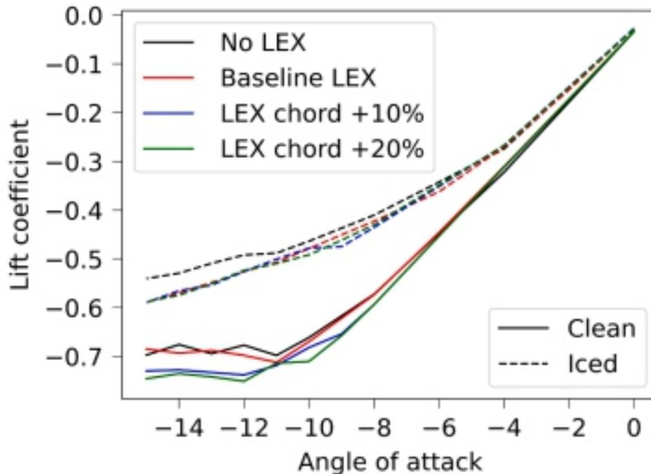
**Fig. 27.**  $C_L$ - $\alpha$  curves for the clean and iced  $10^\circ$  FSHTs with no LEX, baseline LEX, plus 10 % chord LEX, and plus 20 % chord LEX.
