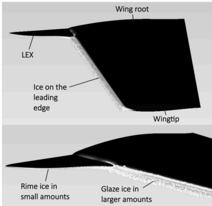
**Fig. 10.** 45-minute ice shape on the FSHT with LEX. This figure has been reprinted with permission from [18], © 2023 SAE International.
