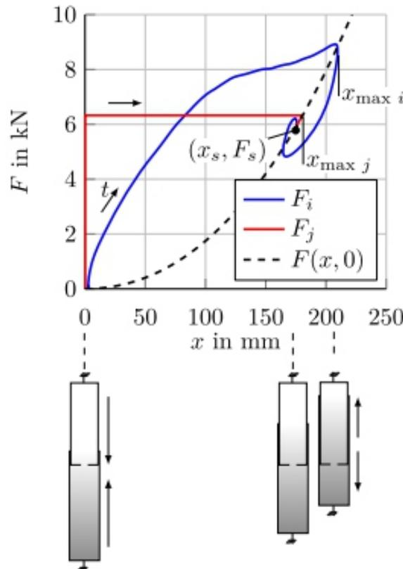
**Fig. 4.** Comparison of ideal energy absorption (red line) during touchdown with that of a non-ideal one (blue line). (For interpretation of the colors in the figure(s), the reader is referred to the web version of this article.)
