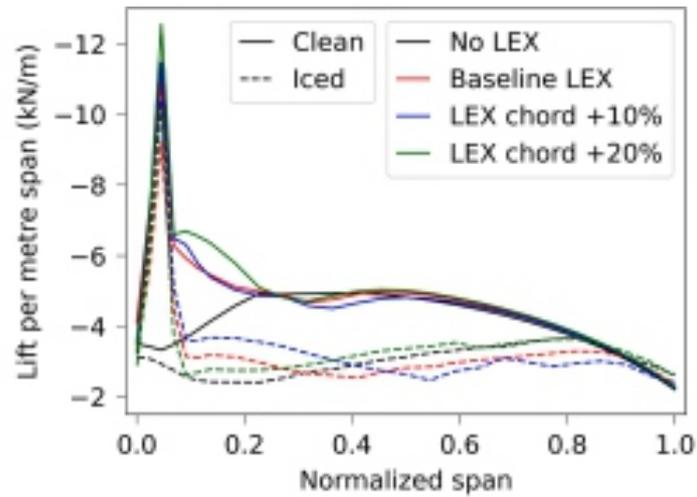
Fig. 31. Spanwise distribution of lift in the form of the integral of streamwise surface static pressure cuts, at  $-10^\circ$  AoA.
