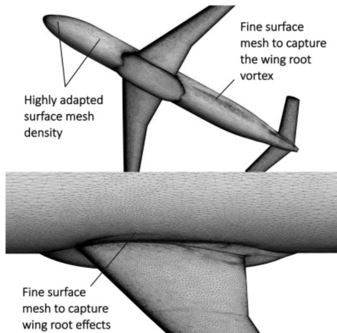
**Fig. 6.** The results of anisotropic adaptation of the aircraft surface mesh based on the air and droplet flow solutions. This figure has been adapted with permission from [18], © 2023 SAE International.
