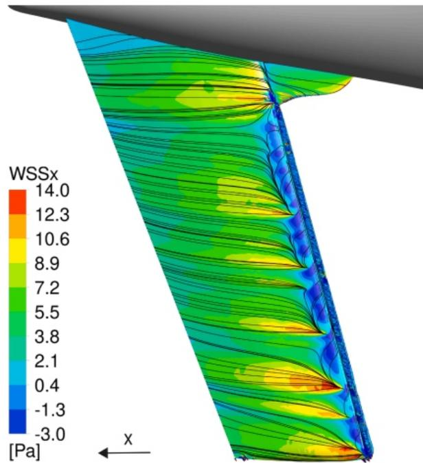
Fig. 15. Iced 15° FSHT suction (lower) surface WSS<sub>x</sub> colour plot with surface WSS vector-based streamlines, at 0° AoA. This figure has been adapted with permission from [18], © 2023 SAE International.
