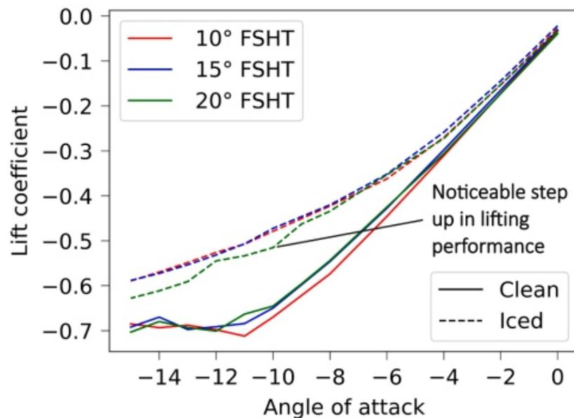
**Fig. 11.**  $C_L$ - $\alpha$  curves for the clean and iced FSHTs with 10°, 15°, and 20° forward sweep.
