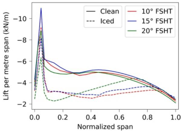
Fig. 22. Spanwise distribution of lift in the form of the integral of streamwise surface static pressure cuts, at -10° AoA.
