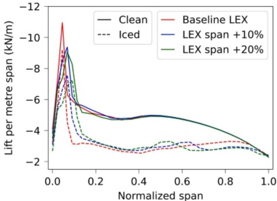
**Fig. 40.** Spanwise distribution of lift in the form of the integral of streamwise surface static pressure cuts, at  $-10^\circ$  AoA.
