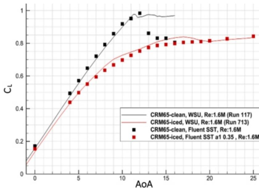
**Fig. 3.** Comparison between Fluent-calculated and experimental  $C_L$ - $\alpha$  curves for the clean and iced CRM65  $37^\circ$  swept wing at a Reynolds number of 1 million and Mach 0.18. This figure has been reprinted with permission from [29], © 2023 SAE International.
