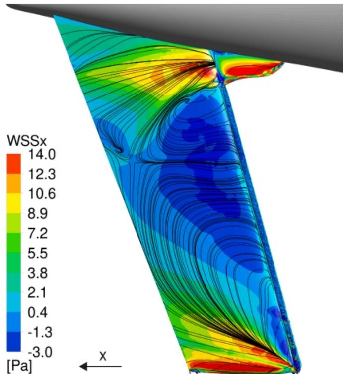
Fig. 19. Iced 15° FSHT suction (lower) surface WSS<sub>x</sub> colour plot with surface WSS vector-based streamlines, at -8° AoA. This figure has been adapted with permission from [18], © 2023 SAE International.
