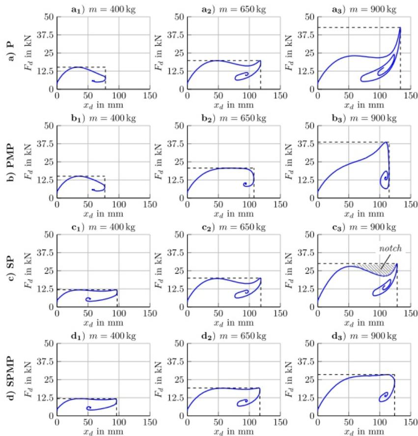
Fig. 11. Comparison of the shock absorber variants P, PMP, SP, and SPMP for a drop mass of  $m = 400$  kg,  $650$  kg, and  $900$  kg at a sink speed of  $v_s = 1.5 \text{ m} \cdot \text{s}^{-1}$  and a ground speed of  $v_g = 25 \text{ m} \cdot \text{s}^{-1}$ .
