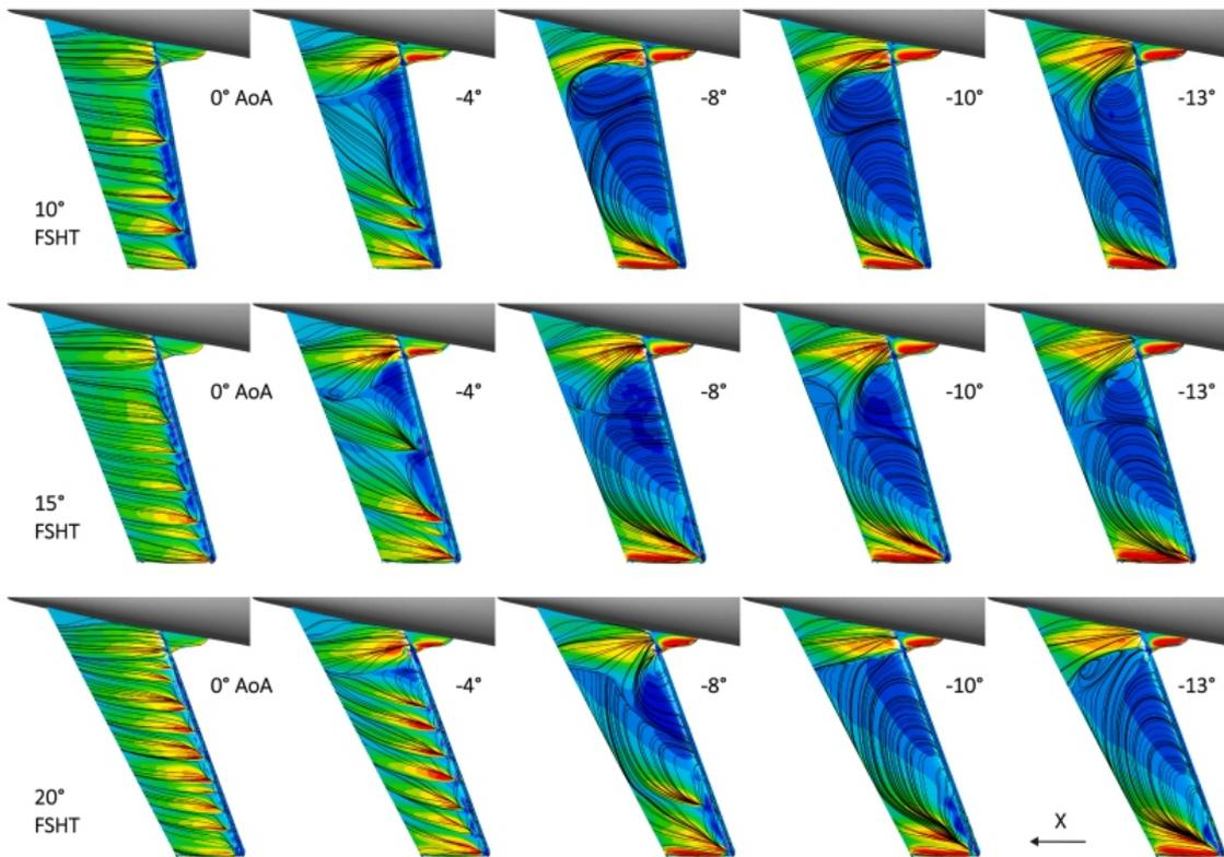
Fig. 21. Suction (lower) surface  $WSS_x$  colour plot, with the same scale as Fig. 18 to Fig. 20, with surface  $WSS$  vector-based streamlines. The rows are iced 10°, 15°, and 20° FSHTs. The columns are 0°, -4°, -8°, -10°, and -13° AoA. The 0° and -8° AoA results have already appeared in different format in reference [18].
