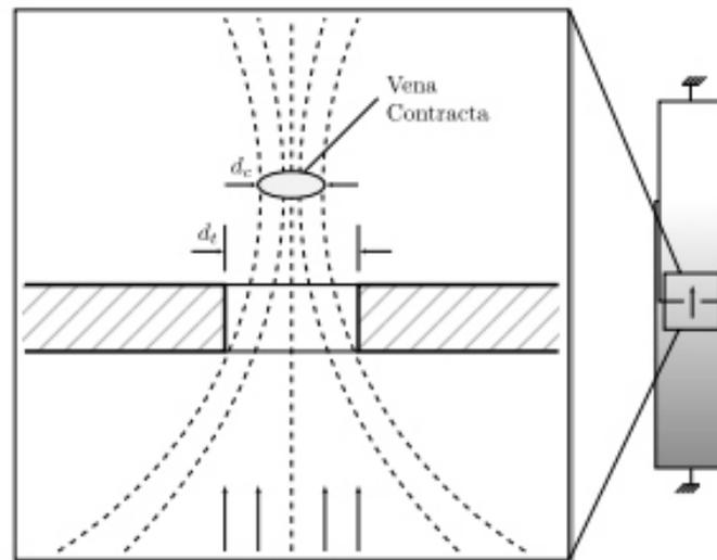
**Fig. 10.** Flow behavior at the throttle.
