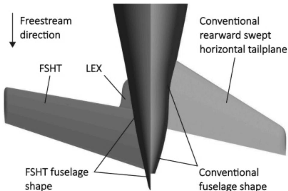
**Fig. 1.** FSHT with LEX geometry with a  $10^\circ$  forward swept leading edge (left) and the conventional reference geometry (right).
