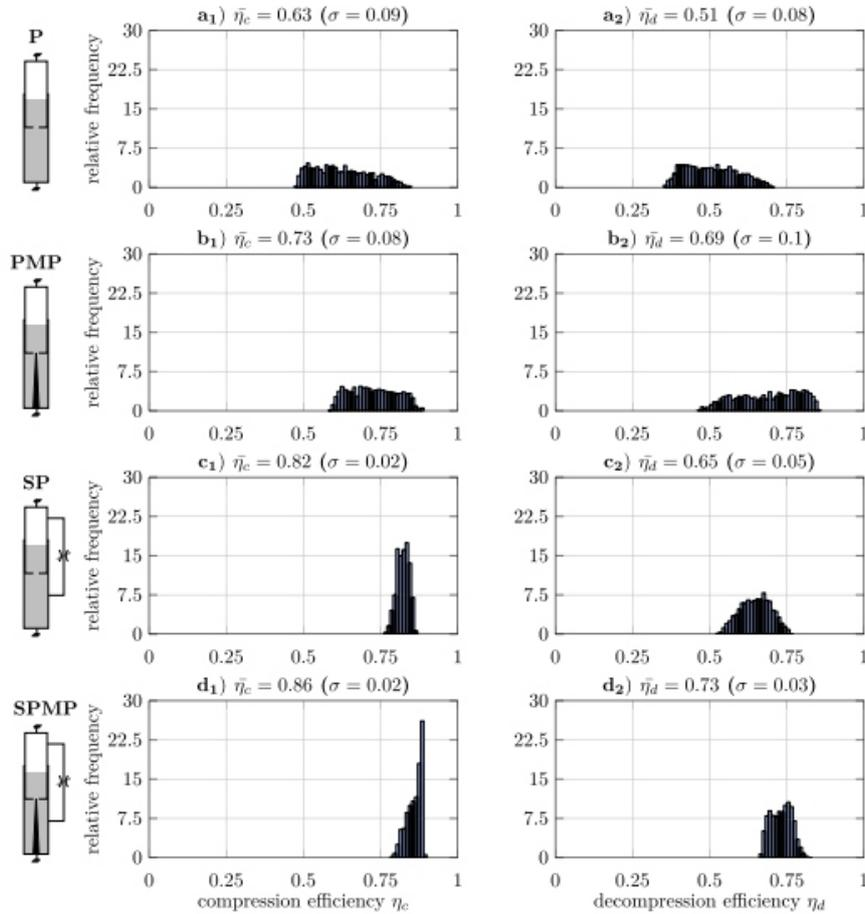
Fig. 13. Compression and decompression efficiencies (binwidth 0.01) as a histogram over a total of 2,067 critical load scenarios in a drop test mass range of  $m = 650\text{...}900\text{ kg}$ , sink speed range of  $v_s = 1\text{...}1.5\text{ m} \cdot \text{s}^{-1}$  and ground speed range of  $v_g = 25\text{...}30\text{ m} \cdot \text{s}^{-1}$ .
