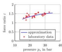
Fig. 7. Ratio between the stationary damping force and total weight force acting on the shock absorber as a function of stationary gas pressure.
