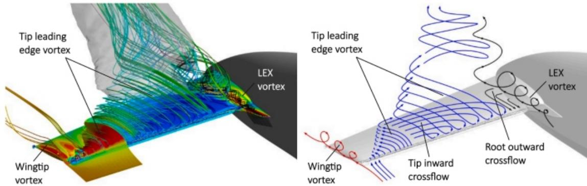
Fig. 25. Iced FSHT CFD-calculated streamlines (left) and corresponding schematic diagram (right) showing the dominant suction (lower) surface flow mechanisms at medium to large negative AoA. Note: the image presents the FSHT suction surface as if it were the upper surface for ease of viewing.
