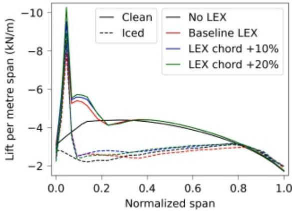
Fig. 29. Spanwise distribution of lift in the form of the integral of streamwise surface static pressure cuts, at  $-8^\circ$  AoA.
