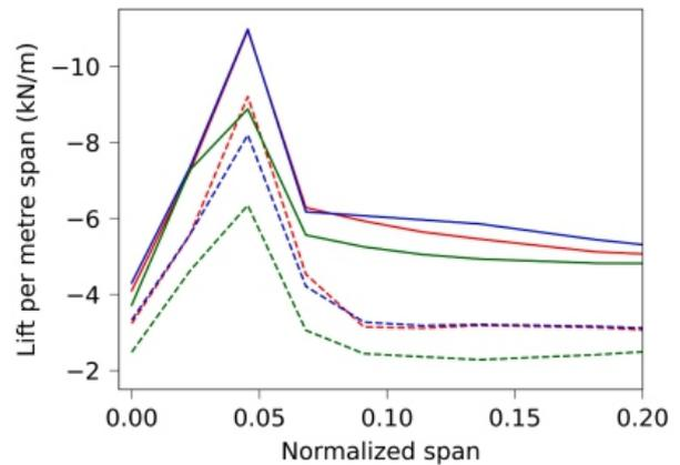
Fig. 23. Spanwise distribution of lift in the form of the integral of streamwise surface static pressure cuts, at -10° AoA.
