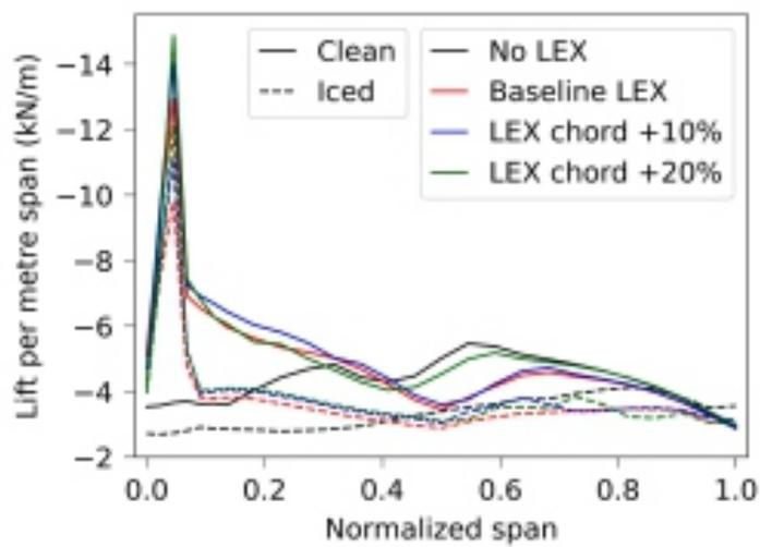
Fig. 33. Spanwise distribution of lift in the form of the integral of streamwise surface static pressure cuts, at  $-13^\circ$  AoA.
