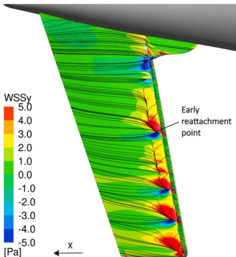
**Fig. 14.** Iced  $10^\circ$  FSHT suction (lower) surface  $WSS_Y$  colour plot with surface  $WSS$  vector-based streamlines, at  $0^\circ$  AoA.
