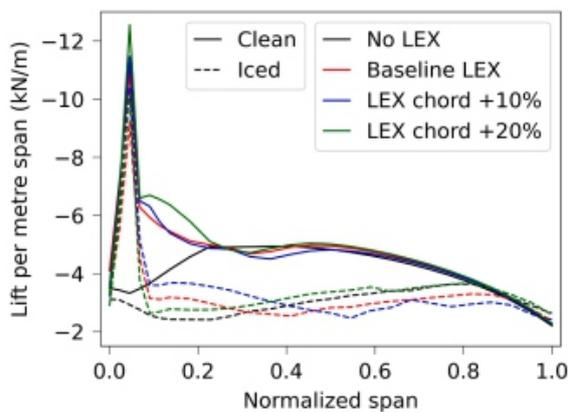
Fig. 31. Spanwise distribution of lift in the form of the integral of streamwise surface static pressure cuts, at  $-10^\circ$  AoA.
