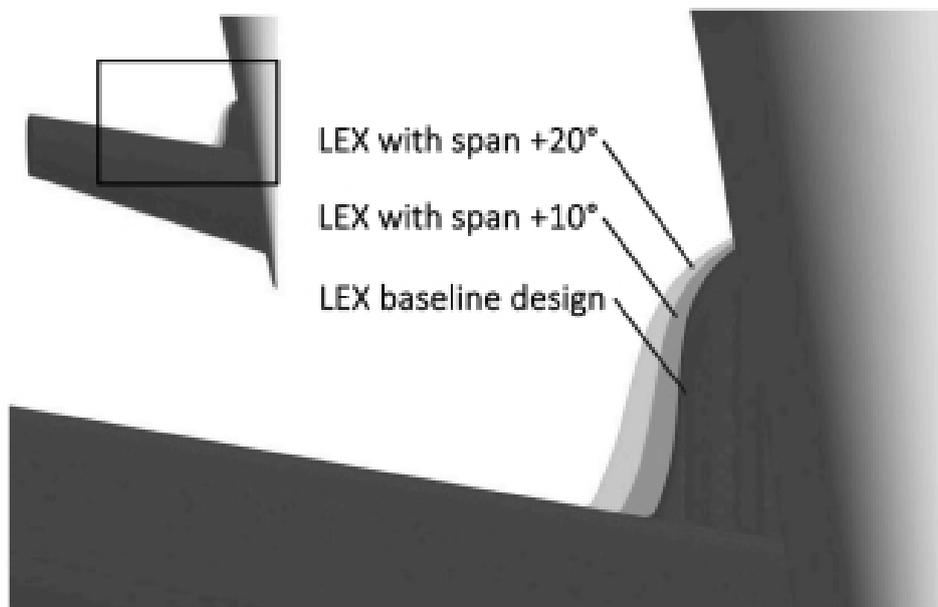
Fig. 35. LEX spanwise geometry variations baseline, plus 10 % span, and plus 20 % span.
