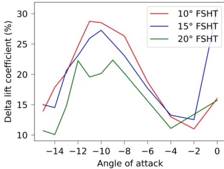
**Fig. 12.** Reduction in absolute  $C_L$  due to ice, expressed as a percentage of clean  $C_L$ , for the FSHTs with 10°, 15°, and 20° forward sweep.
