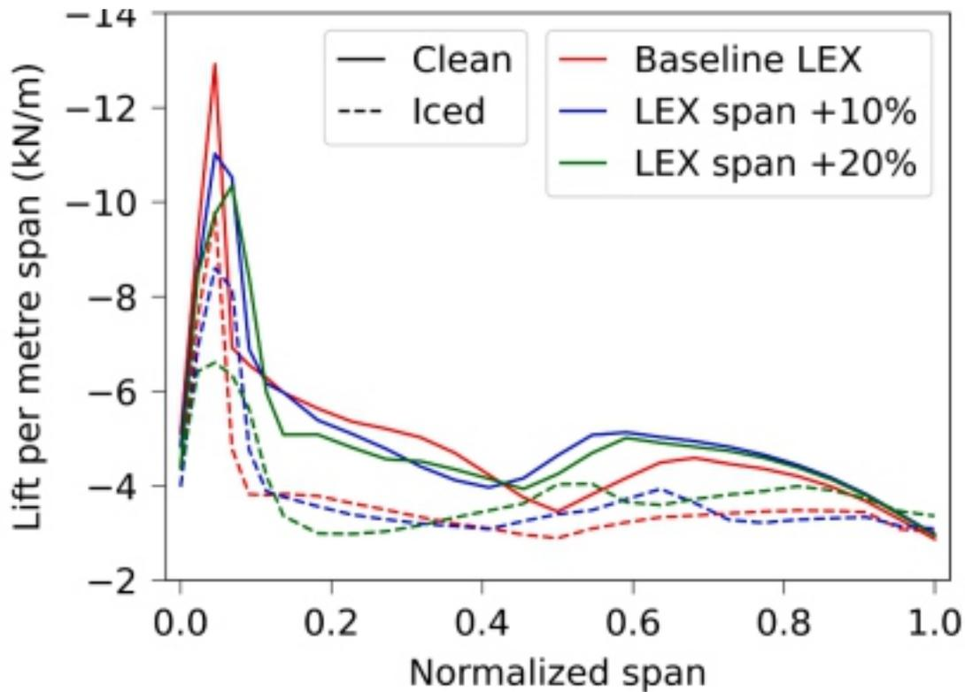
**Fig. 41.** Spanwise distribution of lift in the form of the integral of streamwise surface static pressure cuts, at  $-13^\circ$  AoA.
