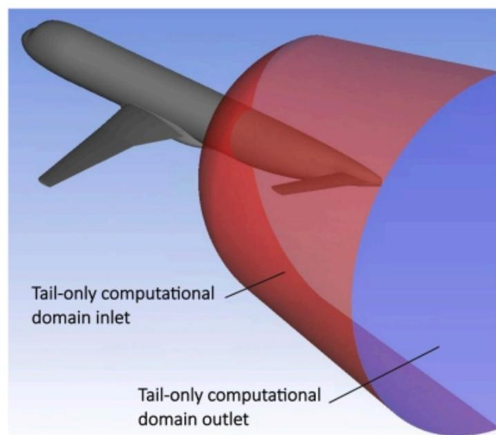
**Fig. 4.** The tail-only domain used for multishot icing simulations of the horizontal stabilizer, with the inlet and outlet boundaries annotated. This figure has been adapted with permission from [18], © 2023 SAE International.
