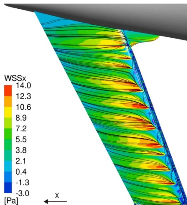
Fig. 16. Iced 20° FSHT suction (lower) surface WSS<sub>x</sub> colour plot with surface WSS vector-based streamlines, at 0° AoA. This figure has been adapted with permission from [18], © 2023 SAE International.
