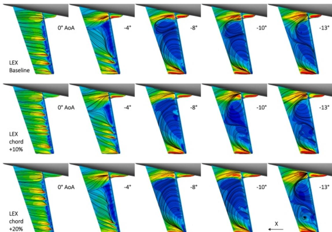
**Fig. 28.** Suction (lower) surface  $WSS_x$  colour plot, with the same scale as used throughout this paper, with surface  $WSS$  vector-based streamlines. The rows are the iced  $10^\circ$  FSHTs with baseline, plus 10% chord, and plus 20% chord LEXs. The columns are  $0^\circ$ ,  $-4^\circ$ ,  $-8^\circ$ ,  $-10^\circ$ , and  $-13^\circ$  AoA.
