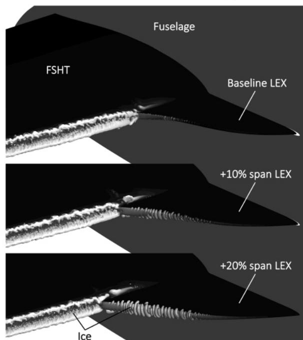
Fig. 36. 45-minute ice shapes on the baseline, plus 10 % span, and plus 20 % span LEXs.
