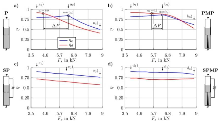
Fig. 12. Compression and decompression efficiencies as a function of the drop load for a sink speed of  $v_s = 1.5 \text{ m} \cdot \text{s}^{-1}$  and a ground speed of  $v_g = 25 \text{ m} \cdot \text{s}^{-1}$  for the shock absorber variants P, PMP, SP, and SPMP, whereby  $v_s$  and  $v_g$  are held constant.
