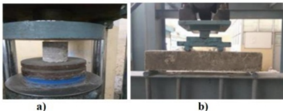
Fig.8. (a & b) Compressive and Flexural testing
