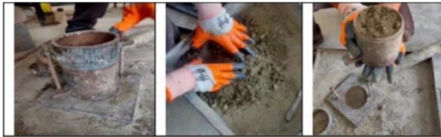
Fig.5. Concrete compaction carried out by Proctor Method for OMC-MDD purpose.
