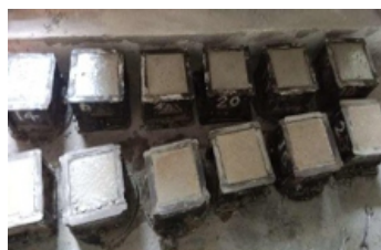
Fig 3. Preparation of moulds
