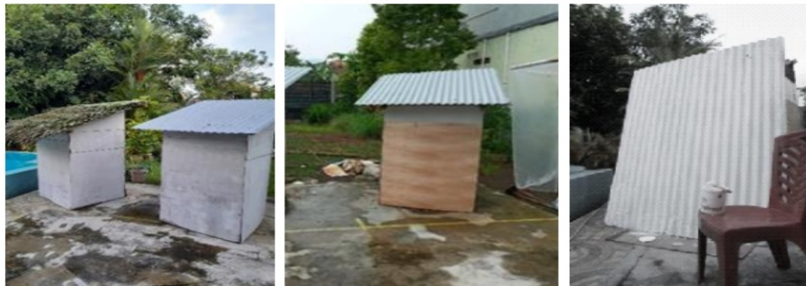
Figure 4. Different roof materials on three test models
