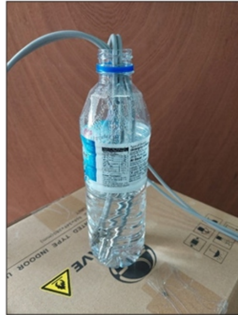
Figure 7. Temperature sensor calibration check in water medium
